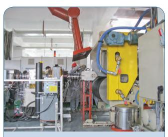
TSE with a gear pump feeding a die in a flat-film/sheet process.
