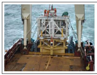
Subsea boosting is emerging as a major growth area for multiphase pumping, and is a key driver for future advancements in multiphase technology. A sharp rise is expected in subsea multiphase boosting installations in deep- and ultradeepwater fields, some of which cannot be produced without boosting from the first day of production. This photo shows a pump as it is being prepared for deplovment in subsea service.
