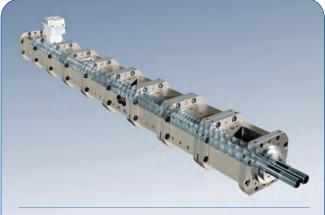
Co-rotating twin-screw extruders utilize segmented screws, assembled on high-torque splined shafts, and modular barrels with internal liquid-cooling bores.
