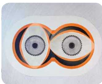
Increased screw volume at the same centreline distance like the ZSE HP series (orange = increase in volume)
