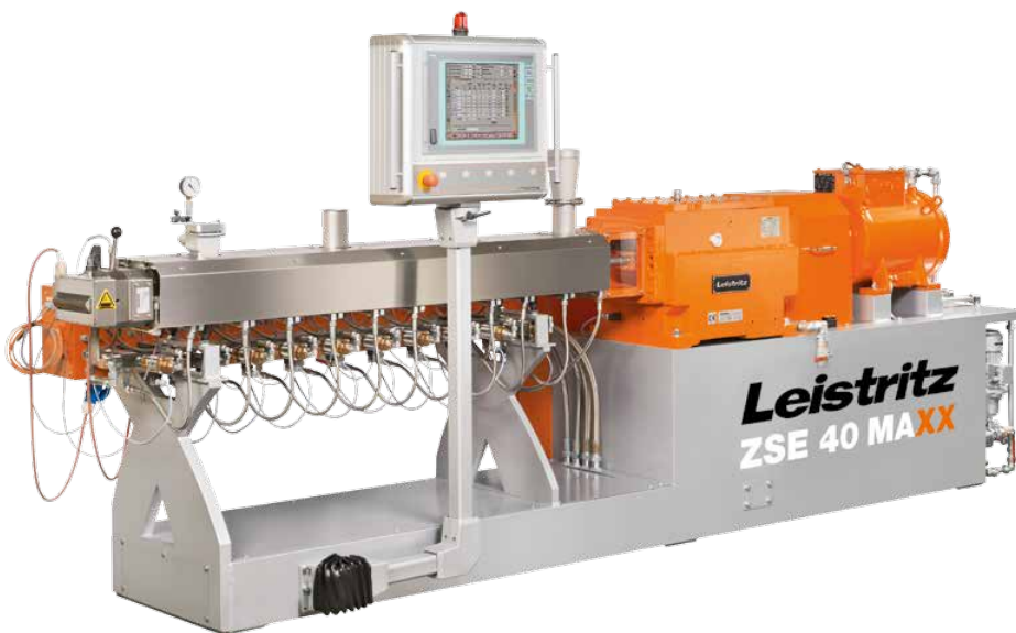
ZSE 40 MAXX - ideal for masterbatch production with throughputs of up to 500 kg/h (depending on the application)
