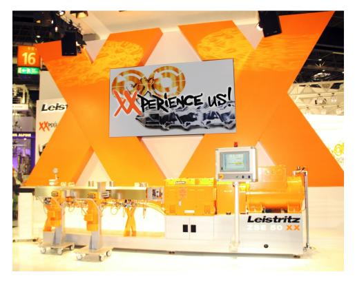
Premiere: The concept extruder ZSE 50 XX with a specific torque of up to 20 Nm/cm<sup>3</sup>
