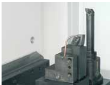
Block toolholder for holding 2 turning tools
