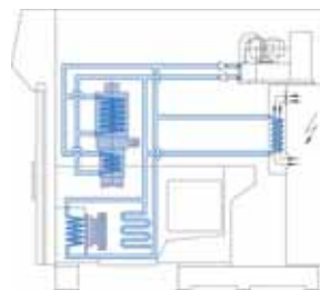
All the machine elements that determine accuracy are connected to the liquid cooling circuit.
