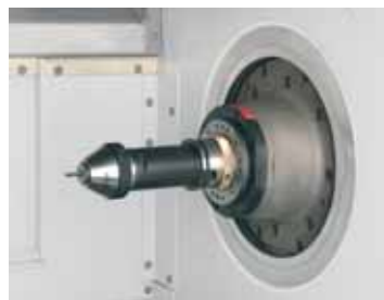
High speed cutting. For milling the recirculation pockets.
