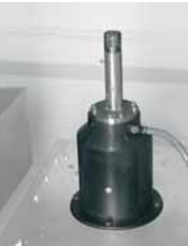
The internal whirling oscillator IWO 100, thermally stabilised
