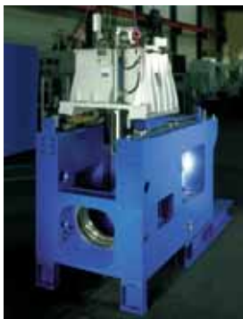
Vibration-damping base of high quality polymer concrete Mineralit ©
