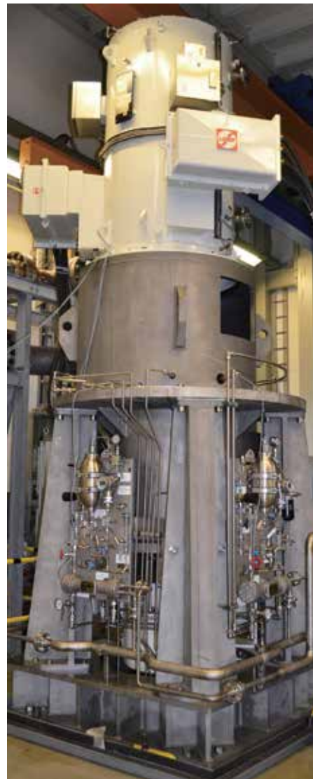
Fig. 5: Vertical Twin Screw Pump as Crude Oil Export Pump for a FPSO
