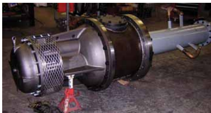
L5NT pump with dip tube components
