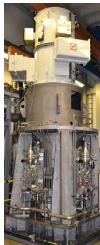
Vertical twin screw pump as crude oil export pump for FPSO
