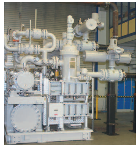
P Multiphase Pump Skid on the Multiphase Pump Test Bed (Photo: Leistriz Pumpen GmbH)
