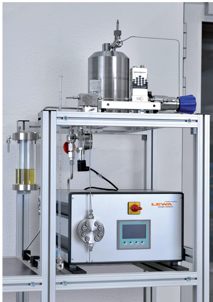
Fig. 2: The high pressure micro-metering pump can provide significantly more precise results under realistic conditions than would be possible with plunger pumps, and is therefore used among other applications for exact, reproducible metering in the processes of high pressure synthesis and high pressure hydration.
