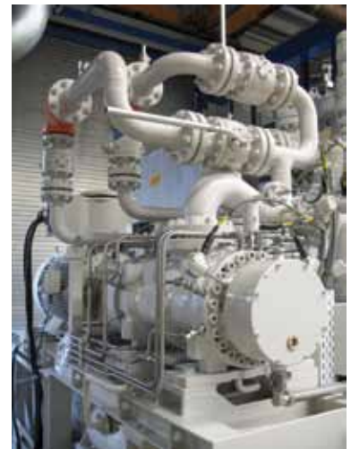
Fig. 5 and 6: Multiphase pump skid on the multiphase pump test bed in Nuremberg
