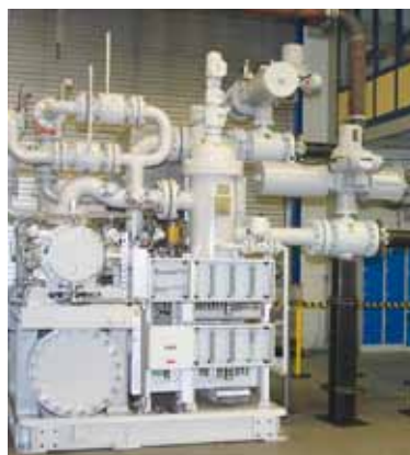
Fig. 5 and 6: Multiphase pump skid on the multiphase pump test bed in Nuremberg
