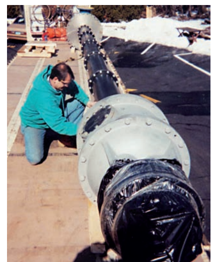
Top picture: Vertical "in-tank installation" of L5NT-Pumps Right picture: Pump and assembly
