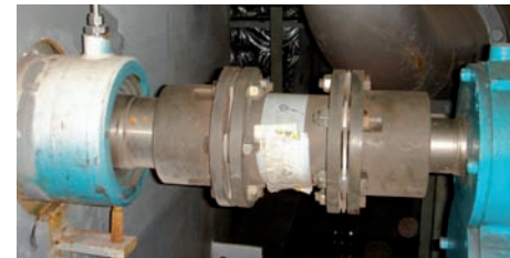
Gastight Bulkhead Seal
