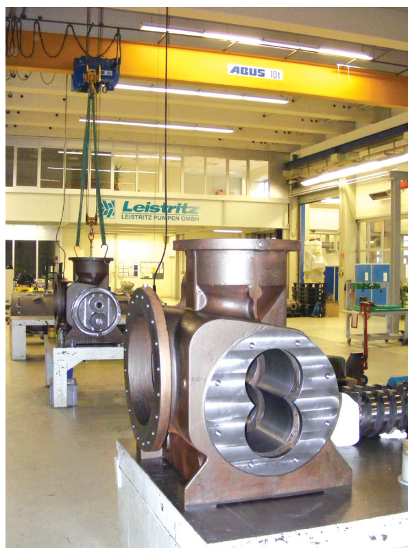
Cargo pumps are employed for loading and unloading oil tankers
