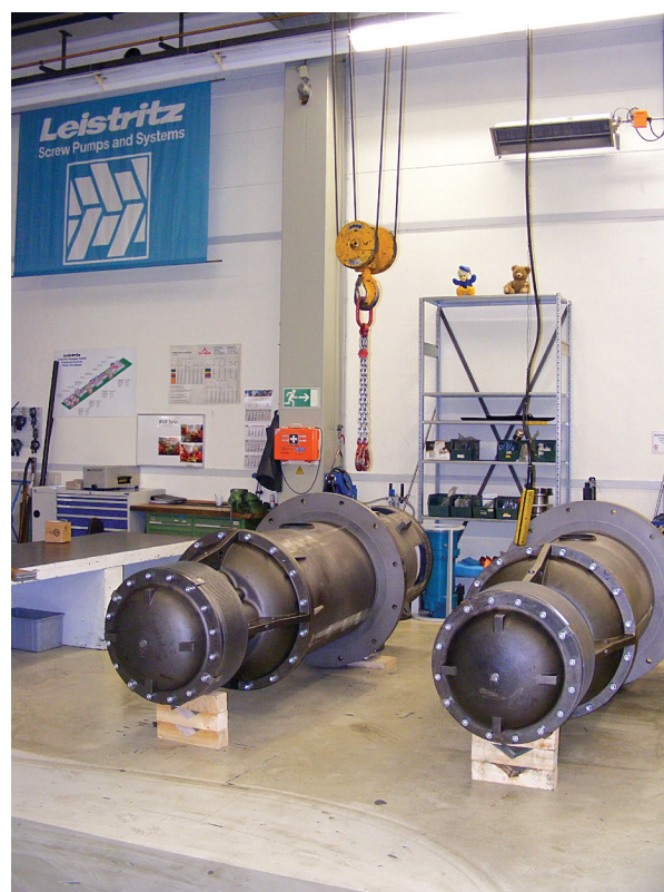
Leistrizt lube oil transfer pumps are used for lubricating marine engines
