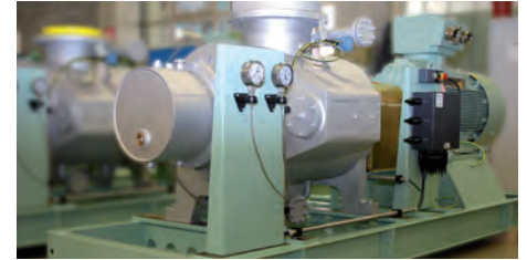
1 Crude Cargo Pump L4NG
