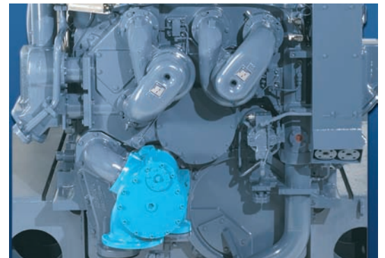
1 Engine driven Main Lube Oil Pump L3NG
