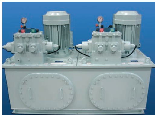
B Tank with Hydraulic Oil Pumps L3MF
